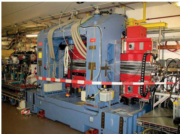
Figure 6.2: Photograph of the UE46 undulator. The magnets are visible as reflective segment between the red painted holding brackets.
