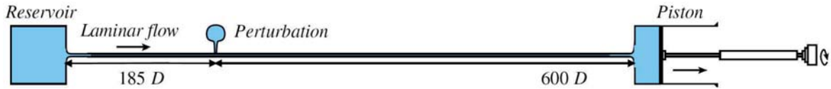
Figure 2.7: Schematic setup of the pipe flow facility for reverse transition investigations. Reprinted with permission from [J. Peixinho and T. Mullin, Physical Review Letters , 96(9):094501, 2006.
