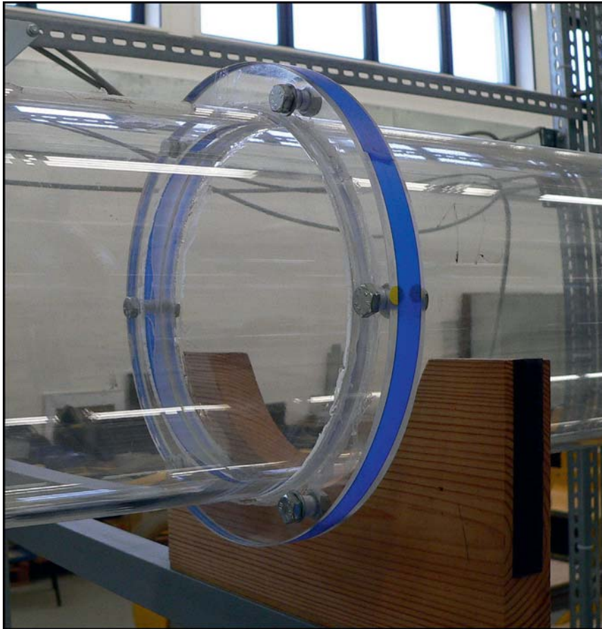
Figure 4.5: Connection of pipe test section through an adhesive bond.
