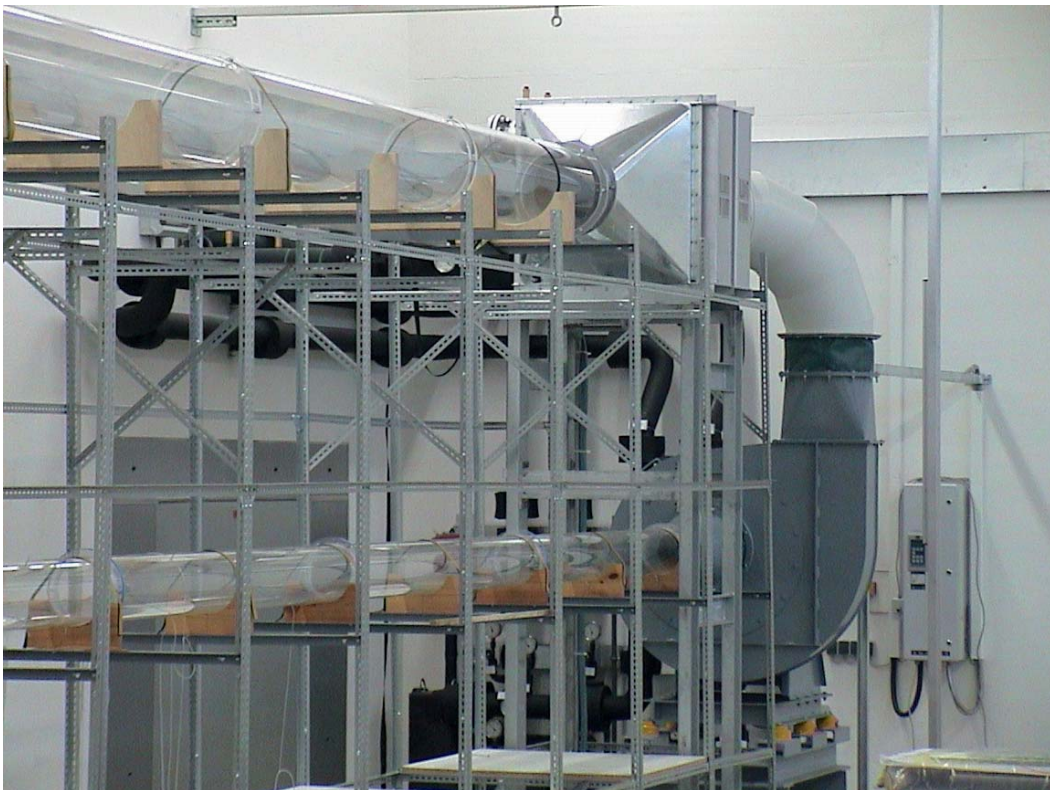
Figure 4.11: Blower and cooling unit with its connection to the return line and actual test section. In the background the mounting of the frequency converter.
