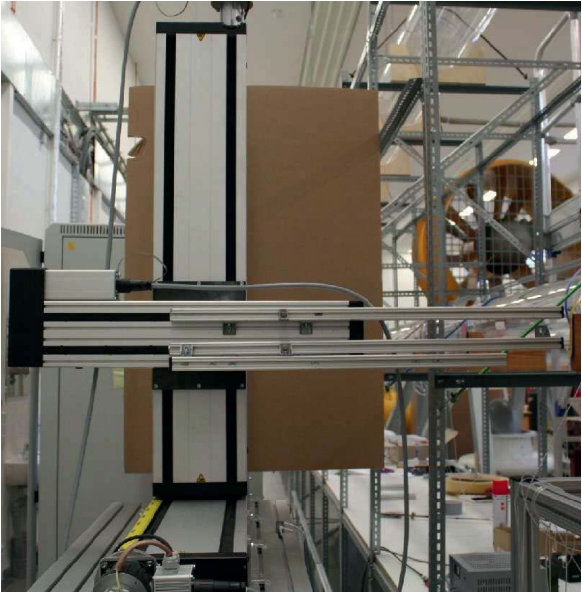
Figure 5.7: Traverse mechanism with independently moving components.
