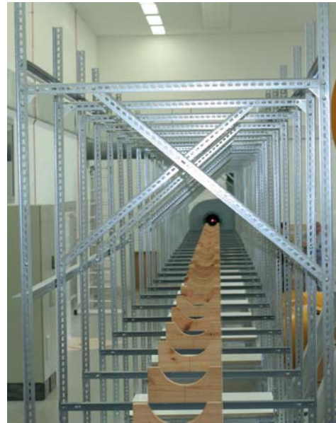
(b) CoLaPipe setup without pipe segments during surveying procedure with the blower unit at the end. The blower unit serves as connection and is therefor the initial point.
