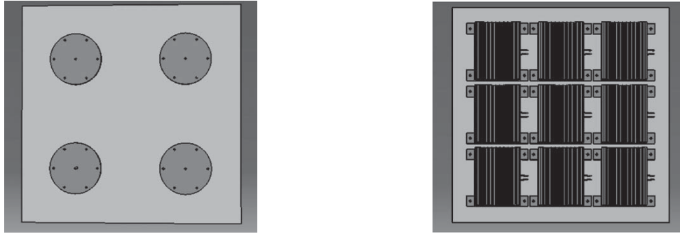
Figure 7.3.: CAD drawing of the heating (left) and cooling plate (right) in the experimental setup of CenCon .
