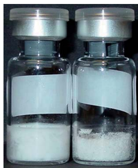
Figure 8.58: Macroscopic appearance of collapsed and non-collapsed PA 01 lyophilizates after storage. Non-collapsed (left) and collapsed (right) lyophilizates after storage at 50 °C for 15 weeks.
