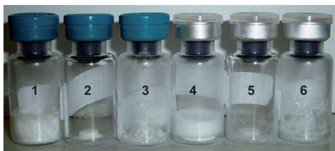
Figure 8.8: Macroscopic appearance of collapsed and non-collapsed lyophilizates stored for 2 weeks at 2 - 8 °C (1 and 4) and 50 °C (2, 3, 5 and 6), respectively.
