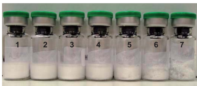
Figure 5.1: Lyophilizates consisting of different ratios of mannitol to sucrose freeze-dried with the collapse-cycle resulting in different degrees of collapse.
