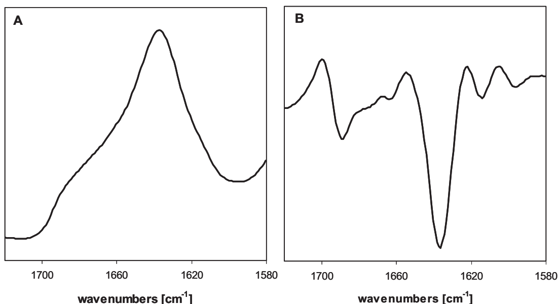
Figure 7.8: FTIR spectra of IgG 01 standard solution in 10 mM sodium succinate buffer pH 5.5: Background corrected, area-normalized amide I FTIR-transmission spectrum (A); area-normalized second derivative amide I FTIR transmission spectrum.
