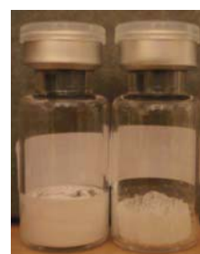
Figure 7.37: Residual moistures and glass transition parameters of collapsed and non-collapsed PA 01 lyophilizates (A), appearance of PA 01 cakes after gentle (left vial) and aggressive (right vial) freeze-drying, respectively (B).
