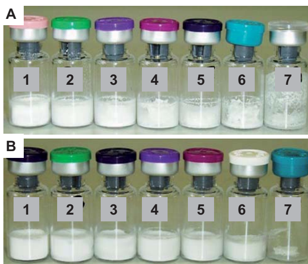
Figure 7.13: Lyophilizates comprising various ratios of mannitol to sucrose freeze-dried using an aggressive drying cycle (A) and a gentle freeze-drying cycle (B), respectively.
