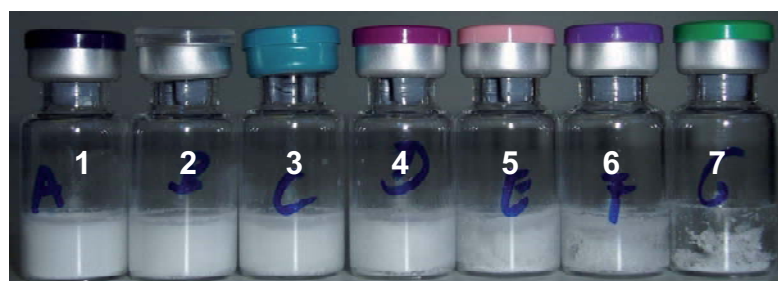
Figure 4.3: Lyophilizates composed of different ratios of mannitol to sucrose (as listed in Table 4.4) aggressively freeze-dried from 10 mM Tris-HCl buffer at pH 7.5 according to protocol 1 (Table 4.3).
