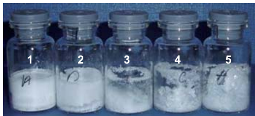
Figure 6.12: Lyophilizates consisting of different ratios of mannitol to sucrose having collapsed to different extents.
