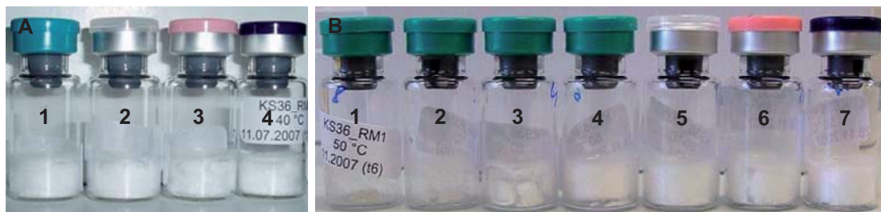
Figure 6.1: IgG01 lyophilizates immediately after freeze-drying with average residual moisture contents of 6.3 % (1), 3.3 % (2), 1.8 % (3) and 0.7 % (4) (A) and after 6 months of storage at 50°C (B) with average residual moisture contents of 6.3 % (1-4), 3.3 % (5), 1.8 % (6) and 0.7 % (7).
