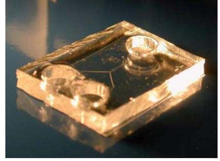
Fig. 4.12: Pressure driven flow: a difference in fluid level between inlet and outlet generates a pressure difference and thus a laminar flow. On the left a schematic of the concept, on the right realization by integrated reservoirs.
