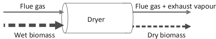
Figure 23: Feed and product mass flows of a direct rotary dryer
