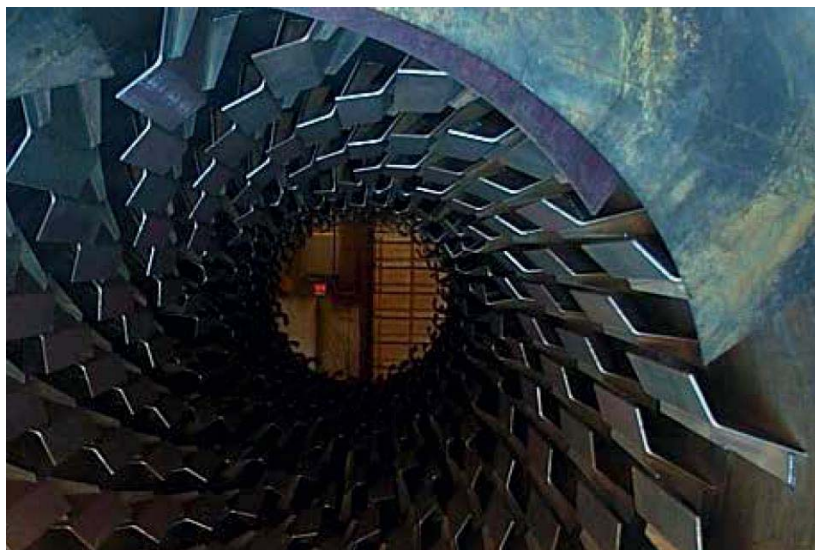
Figure 8: Flights in a direct rotary dryer [60]
