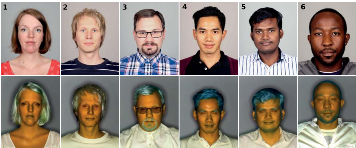
Figure 2.4: Visual spectrum (RGB color) and short wave infrared (false color) portrait images of skin types 1 to 6 according to Fitzpatrick [40].
