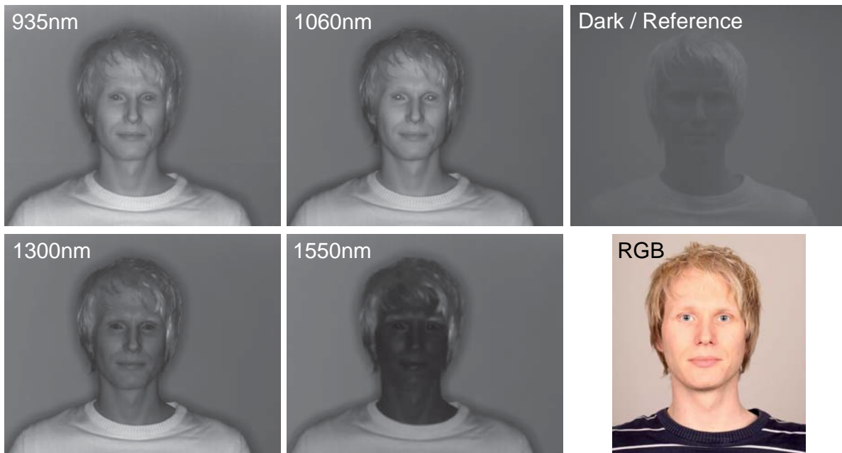
Figure 7.1: The multispectral image cube acquired by the SWIR camera system compared to an RGB color image.
