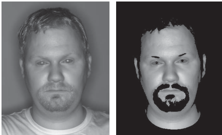
Figure 5.4: SWIR image before (left) and after (right) masking out all non-skin pixels. Previously presented in [22].
