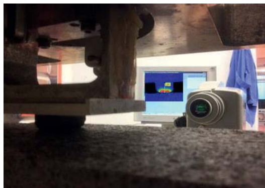
Fig. 5.48: Experimental set-up for the IR thermal camera measurements during sliding friction.
