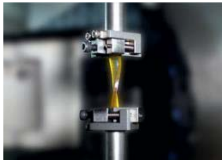
Fig. 4.1: Detail of the sample during a torsion dynamical test performed by the ARES.
