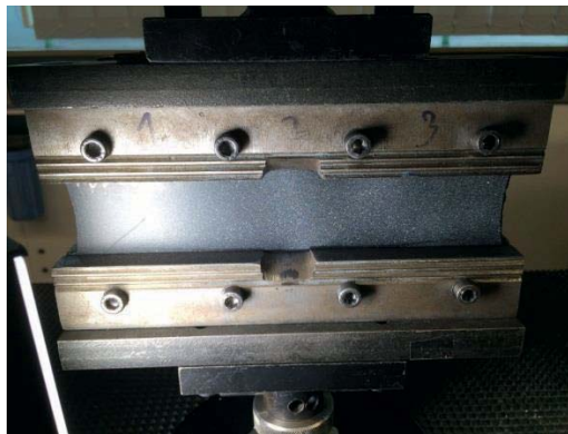
Fig. 4.2: Pure shear test seen from the front. Sample stretched at 30%.
