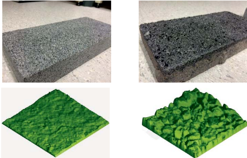
Fig. 5.33: Substrates used for the investigation: granite paver (left side), brick paver (right side). 3D Magnification render for a 10 x 10 mm 2 area on the bottom part.
