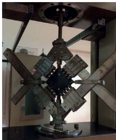
Fig. 4.3: Equi-biaxial test performed in the Zwick machine.
