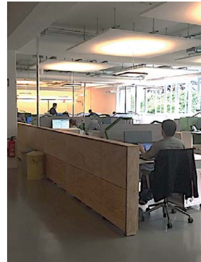
Office IT, vitra Wiring via ceilings and half-height partitions. With the use of textiles, the latter creates zones for infrastructure and meetings
