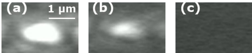
Figure 6.61: Images from the near infra-red camera show the output of the DLSPW waveguides at different polarizations of input light (at  $1.55 \mu\text{m}$  wavelength). (a)  $0^\circ$  Polarization (b)  $45^\circ$  Polarization (c)  $90^\circ$  Polarization. As can be seen, output intensity decreases drastically with polarization.
