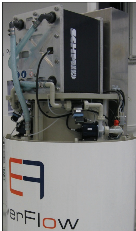
Figure 1-5: 2-kW/10-kWh VRFB prototype by SCHMID Energy Systems GmbH, Freudenstadt, Germany [10]
