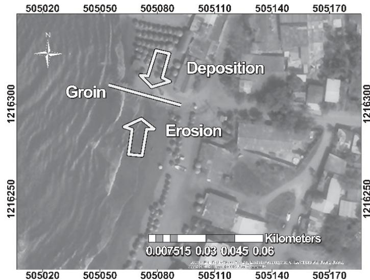
Figure 4: Erosion/sedimentation processes caused by coastal structures.
