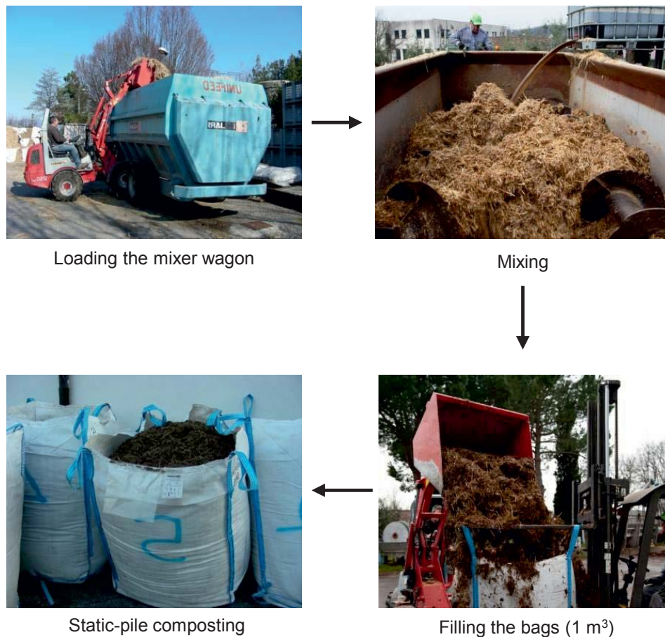
Figure 3.8: Processing of olive-mill waste compost
