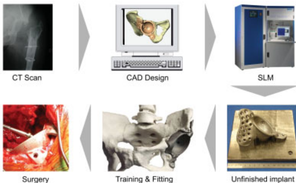
Figure 3.10: Process chain for a customized acetabulum endoprosthesis [254]
