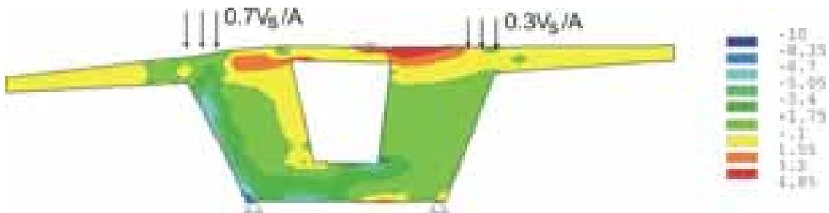
**Figure 3.31** Horizontal stress  $\omega_x$  - inelastic material behaviour
