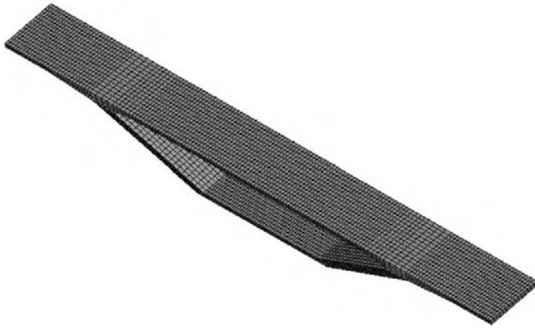
Figure 3.19 Finite element model of a standard segment of Bang Na bridge (~ 9300 brick elements)
