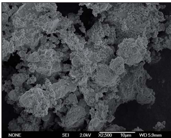
Figure 6: SEM micrographs of (a) primary glass particle fraction ( < 45 \mu\text{m} ) used for adsorption experiments and (b) second fraction used for electrophoretic mobility measurements.
