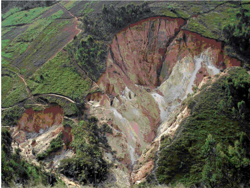
Fig. 5. Artisanal mining of weathered tantalum-rich pegmatite by “ground sluicing” (Kabarore area, northern Burundi). The economic portion of such deposits is only about 500 g per ton ore. The 99.9 % of waste is washed down into the valley where it spills over large areas of fertile soil
