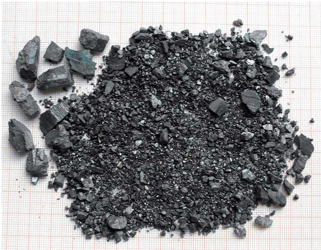
Fig 2. Tantalum ore (“coltan”) consists of the Ta-rich member of the columbite mineral group, (\text{Mn,Fe})(\text{Ta,Nb})_2\text{O}_6 , a black, heavy accessory mineral in rare-metal-rich granite pegmatites
