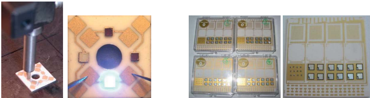
Fig. 2 Realization of specimen for T5 and Baker Hughes: Optoelectronic module consisting of two PDs and LEDs bonded on \text{Al}_2\text{O}_3 -substrate (left) and bonded BC817/Fairchild and SIGC15T60/Infineon on \text{Al}_2\text{O}_3 -substrate for testing at BHI (right).
