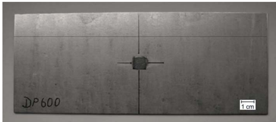
Fig. 12: Specimen for bending tests with dezincified spot in the center
