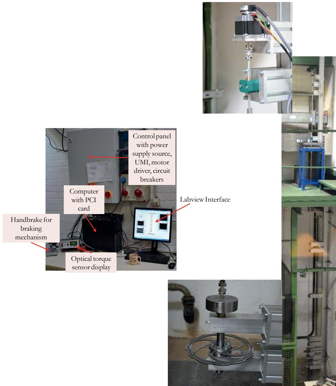
Figure 3. Scheme of the experimental setup to study drill string vibrations
