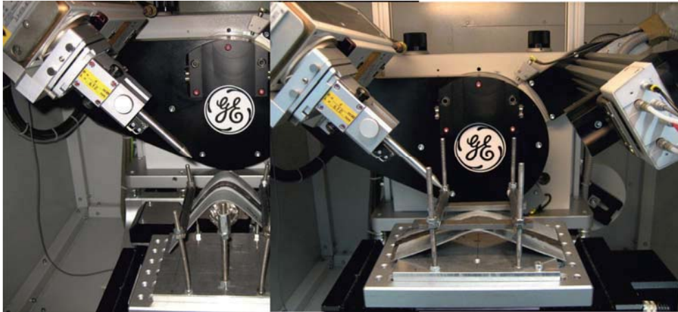
Fig. 22: Device for measuring load stresses during bending and unbending mounted to the Diffractometer
