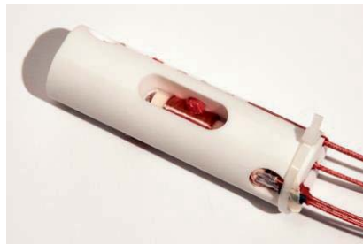
Fig. 10: Completed three-axis fluxgate sensor prior to silicone filling.
