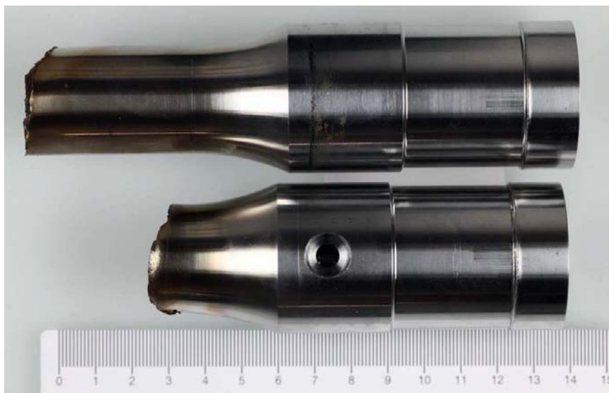
Fig.9: Fractured specimen of alloy P550.
