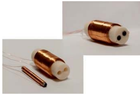
Fig. 9: Individual components of a fluxgate sensor during the assembly process. Left: Bobbin with detection coil and core with excitation coil. Right: Complete, assembled sensor.
