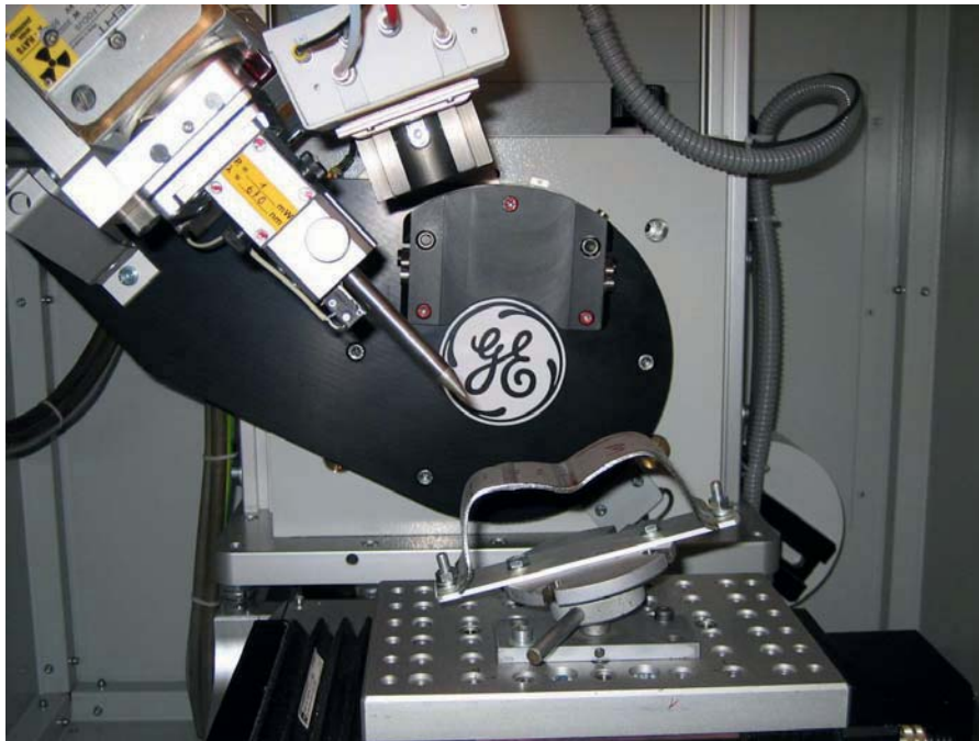
Fig. 24: Device for measuring residual stress at tube segments with suppressed springback
