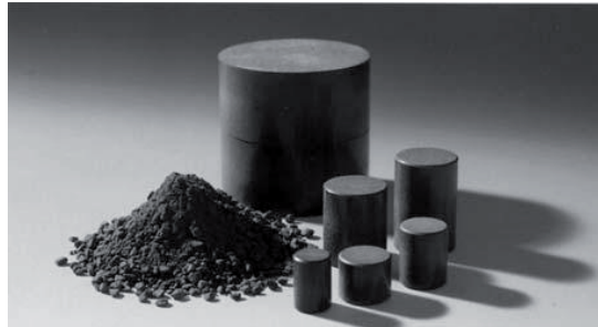
Figure 3.1 Examples of epoxy molding compounds in powder and pellet forms (Komori and Sakamoto, 2009).
