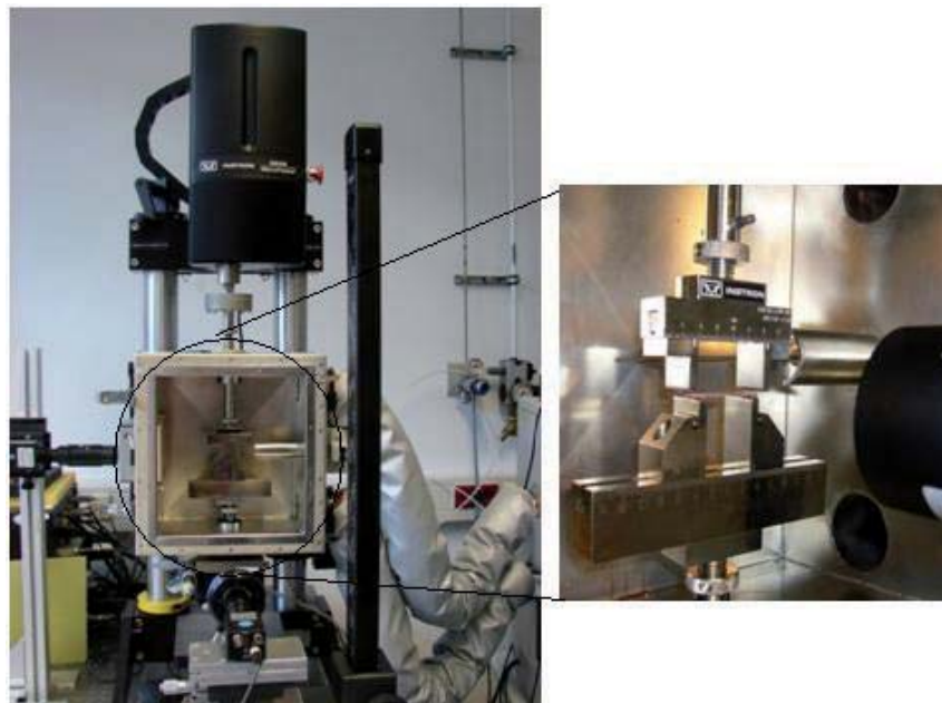
Figure 3.3 The load frame used for the measurement of interfacial fracture toughness (left) and the four-point bend fixtures (right).
