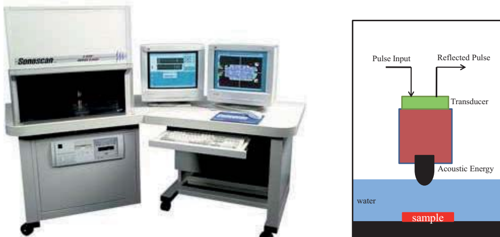
Figure 3.11 C-SAM equipment (left), schematic representation of the C-mode scanning acoustic microscope (right).
