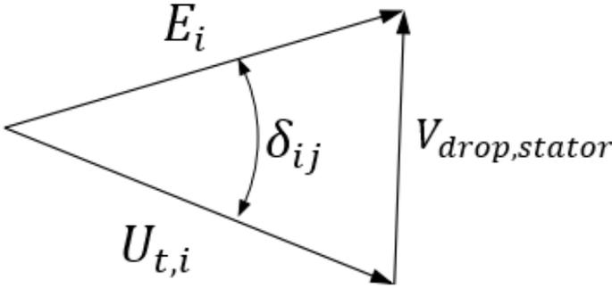
**Figure 4.4.** Virtual voltage drop estimation using cosine law
