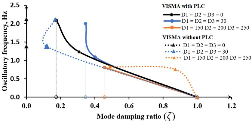
**Figure 6.3.** Impact of damping on system pole locations.
