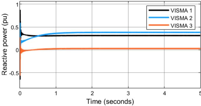
**Figure 4.10.** Reactive power injection at the virtual buses
