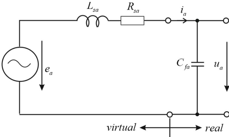
**Figure 2.10.** Per phase equivalent-circuit of ESM (phase a)
