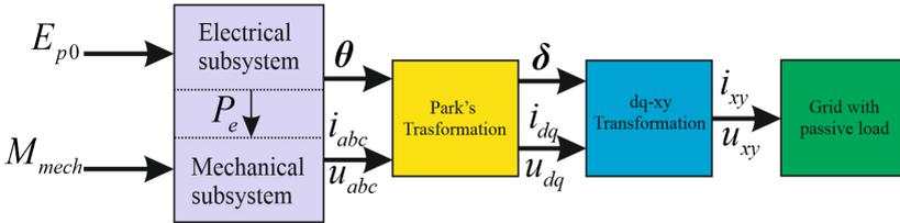
**Figure 5.4.** Stages of the entire system model
