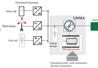
**Figure 1.6.** Basic structure of VISMA [18]
