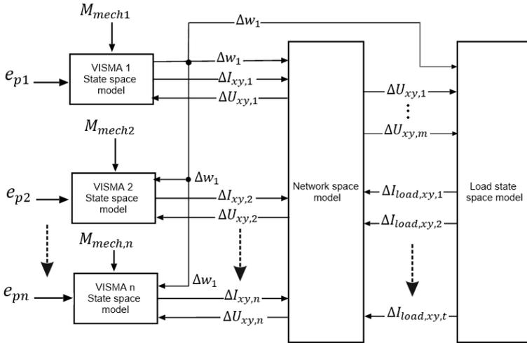
**Figure 5.5.** Complete small-signal model of  $n$ -VISMA microgrid
