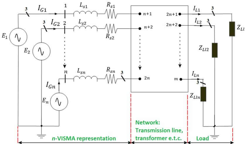
Figure 5.1.  $n$ -VISMA with constant impedance loads
