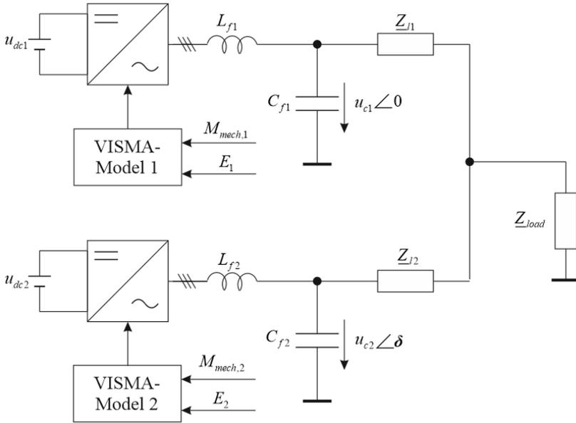
**Figure 4.12.** Two VISMA low voltage model [48]
