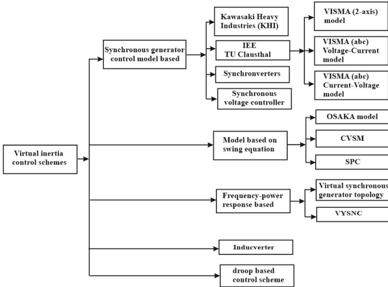
**Figure 2.1.** Virtual Inertia Control Topologies, modified from reference [41]
