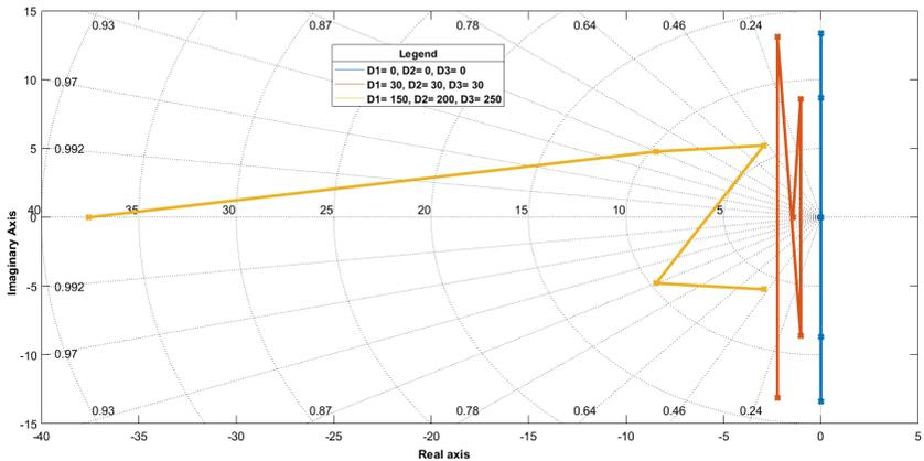
Figure 5.11. Impact of damping on system pole locations
