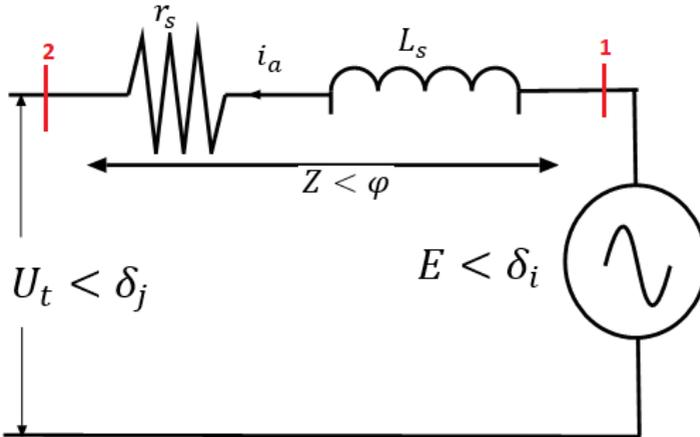
**Figure 4.3.** Per phase equivalent circuit of VISMA stator
