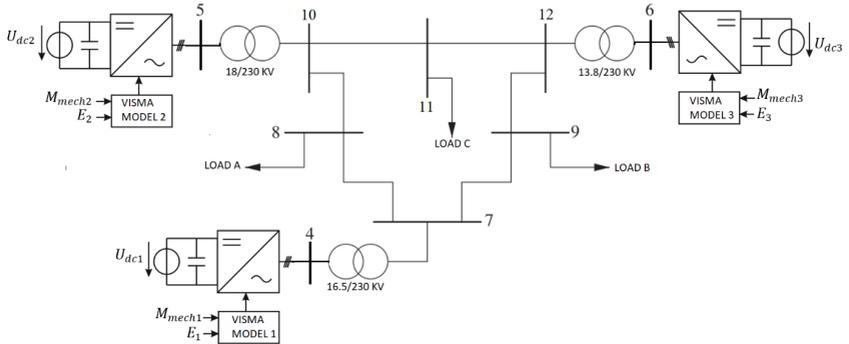
**Figure 3.3.** VISMA model with external power loop control
