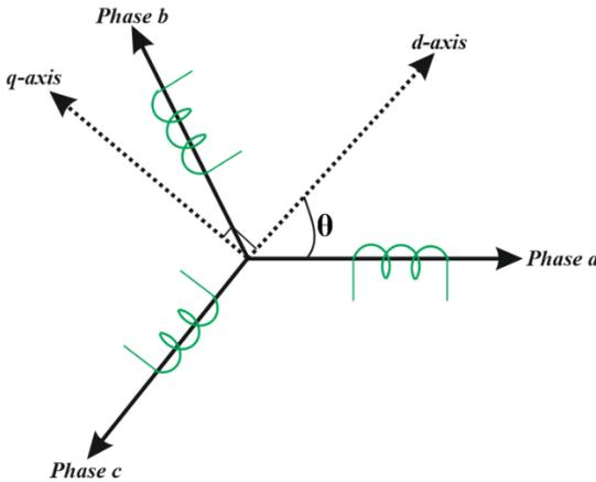
**Figure 2.11.** 3 –  $\phi$  machine and d-q equivalent
