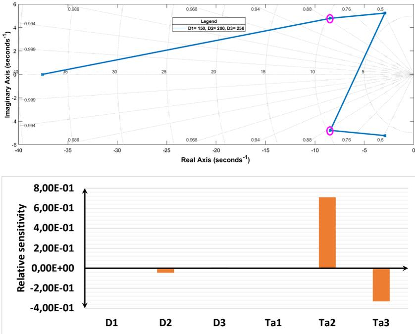
Figure 5.13. Parameter sensitivity of the fastest oscillatory mode
