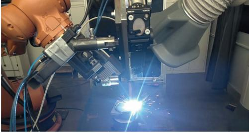
*Abb. 1. Additive welding process with industrial robot.*
