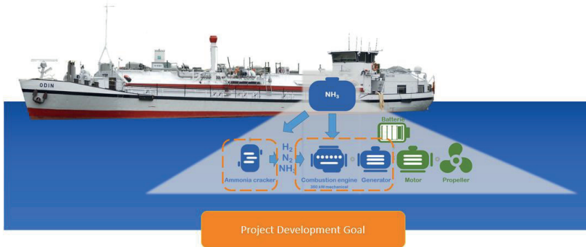
Figure 1: Ammonia based propulsion concept
