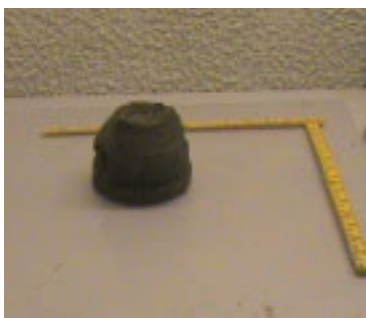
Figure 5.2.1.1.5: Mini slump of mortar produced with high yield cement
