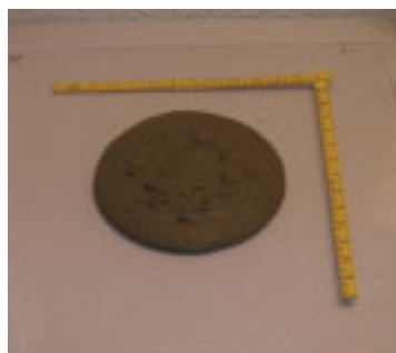
Figure 5.2.1.1.6: Mini slump of mortar produced with intermediate cement
