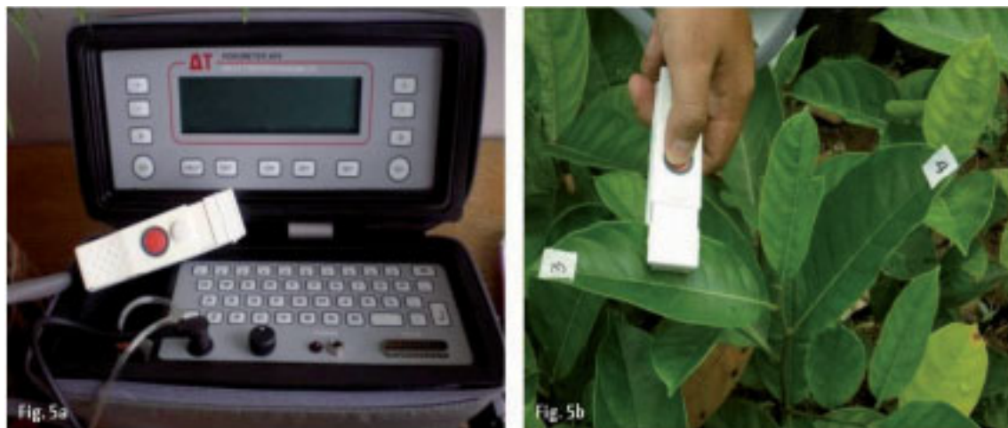
Figure 5 (a) Delta-T Porometer type AP4 (Delta-T Devices Ltd., Cambridge, England, UK) (b) Stomatal conductance measurement on mature leaves of Artocarpus heterophylla in the nursery. Measurements were taken from the widest width of the leaf approximately 1-2 cm from the leaf edge.
