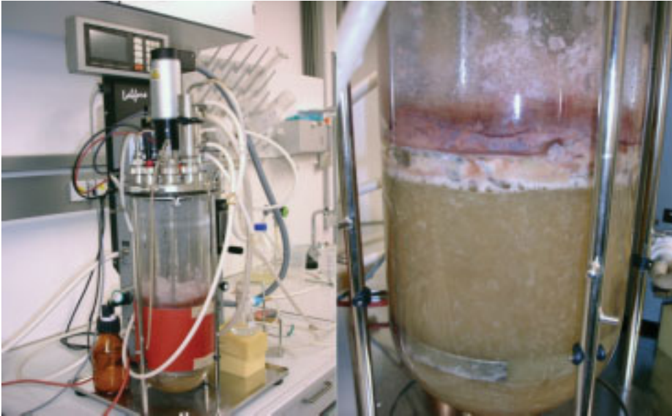
Figure 3.6: Bench-top fermenter, obtained inoculum after three days of fermentation
