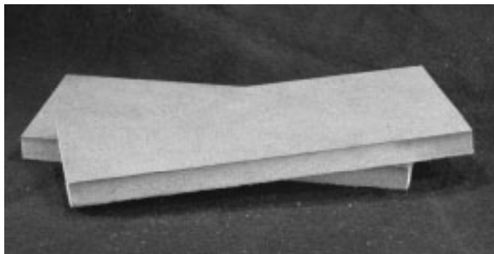
Fig. 2 MDF produced with laccase from Pleurotus ostreatus wheat straw cultures (section 2.II) at the pilot plant for MDFs at the Büsgen Institute, Section Molecular Wood Biotechnology and Technical Mycology
