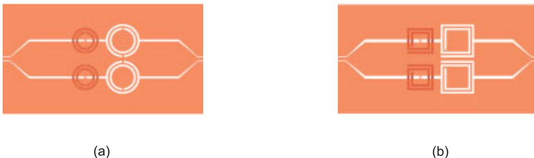
Figure 4.28: Layout of the structure (SRR/SL-CSRR) CPW (a) and the proposed structure (RSR/SL-CRSR) CPW (b), respectively.
