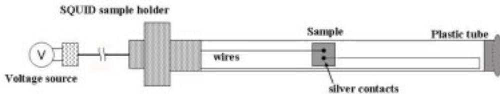
Figure 3.3: Scheme of the sample holder for low-temperature polarization measurements.
