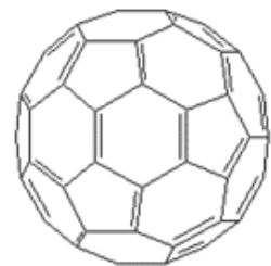
Abb. 7: Das C 60 -Buckminsterfulleren.
