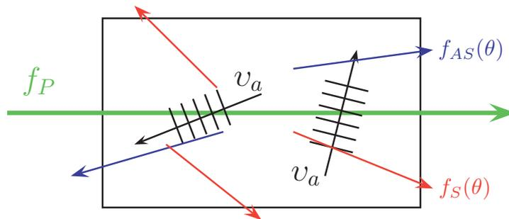
Figure 2.1.: Scattering process of spontaneous Brillouin scattering.
