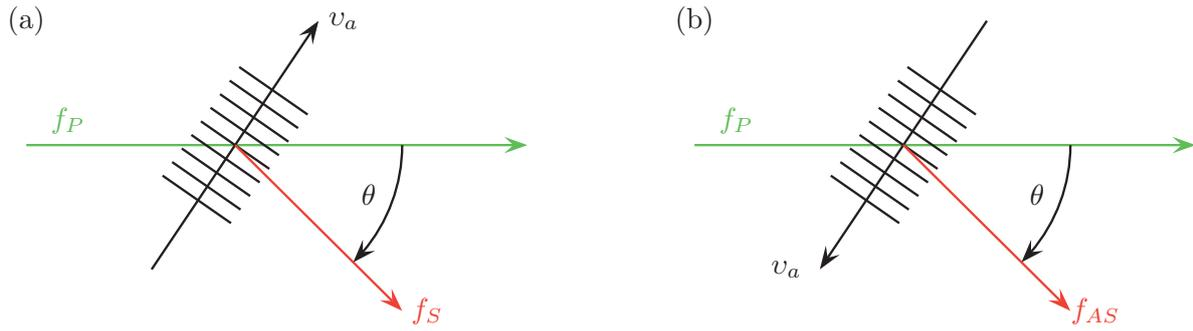
Figure 2.3.: Depending on the propagation direction of the sound wave  $v_a$  with respect to the pump light wave with the frequency  $f_P$ , Brillouin scattering generates at a scattering angle  $\theta$  a Stokes wave (a) with a smaller frequency  $f_S$  or an anti-Stokes wave (b) with a higher frequency  $f_{AS}$  with respect to  $f_P$ .
