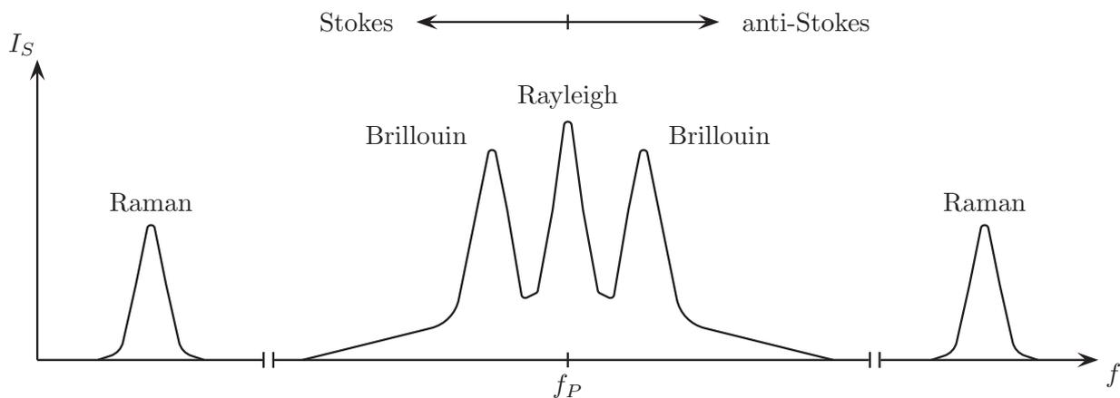
Figure 1.1.: Schematic representation of a typical spectrum of the scattering of light [4].
