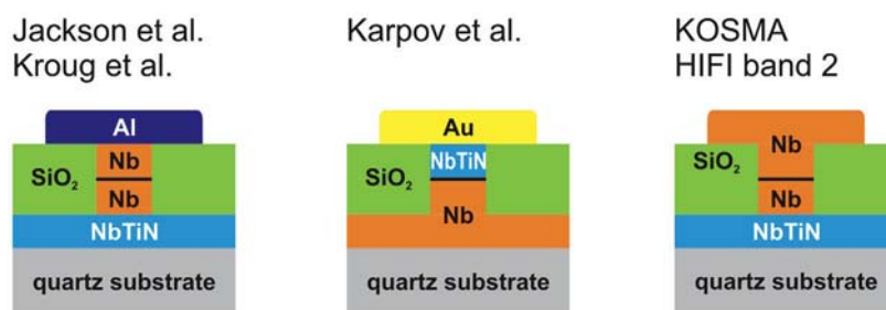
Figure 1.6: State of the art SIS devices. Above 700 GHz the Nb wiring leads can be regarded as normal conducting. These devices have been published in [20, 25–27]
