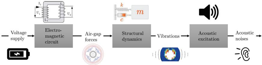
Figure 1.4: Causality chain from voltage excitation to acoustic noises
