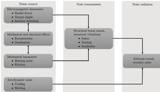
Figure 2.2: Noise sources in electrical drives
