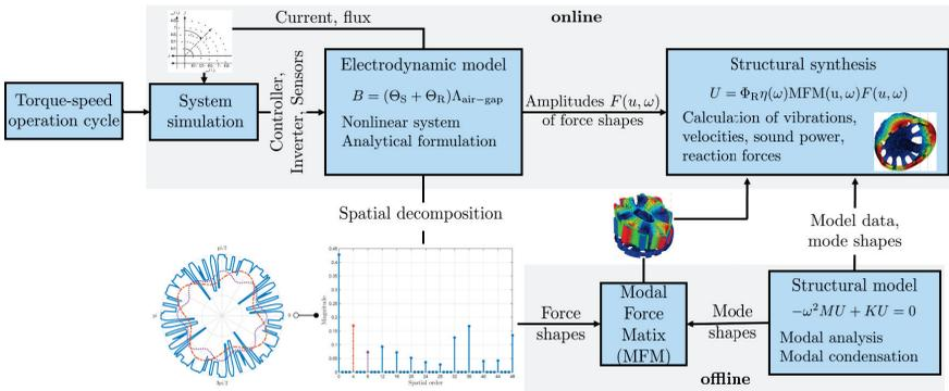
Figure 1.5: Simulation path for efficient NVH simulations (based on [Kot+17b; Boe13])
