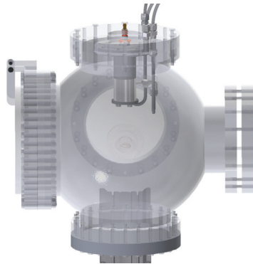
Figure 1.1: INGA III experimental setup with Laval nozzle fixed on the top lid of the spherical vacuum chamber.
