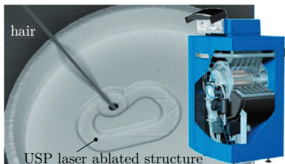
Fig. 1.1 SEM image of a spray nozzle plate (left) used in oil burners for heating systems (right). A human hair is presented for a better visualization of dimensions. The inner structure is ablated by means of USP lasers at Bosch production sites [8].
