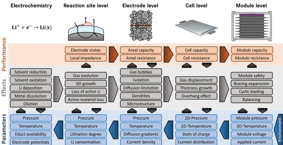
**Figure 1.1** Complexity diagram for lithium-ion battery aging interacting on different scales. Effects can have backtracking effects by changing parameters and affect performance. Concept explanations will follow in this thesis.
