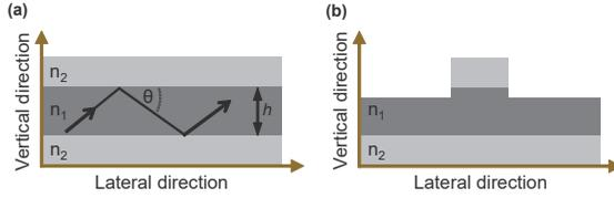
**Figure 2.1:** Schematic representation of (a) a vertical slab waveguide with  $n_1$  and  $n_2$  being the waveguide core and cladding refractive indices, respectively. Panel (b) shows a RW which can be formed by selectively removing parts of the slab waveguide.
