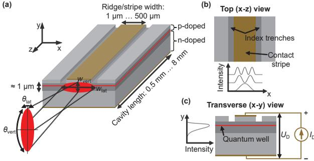
**Figure 1.1:** Schematic (a) three-dimensional representation of an edge-emitting diode laser including information on typical device extensions. In addition, the resulting radiation behavior including its defining parameters is shown. Panel (a) and (b) show the corresponding lateral-longitudinal ( $x$ - $z$ ) top view and a lateral-vertical ( $x$ - $y$ ) transverse cross-section, respectively.
