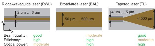
**Figure 1.2:** Schematic top view of a ridge-waveguide laser (RWL), a broad-area laser (BAL), and a tapered laser (TL). Underneath each laser type a rough classification in terms of beam quality, electro-optical efficiency, and optical output power is given.
