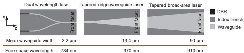
**Figure 1.3:** Schematic top view of the three investigated lateral-longitudinal non-uniform laser cavity designs. In addition, the corresponding mean waveguide widths and emission wavelengths are summarized at the bottom.
