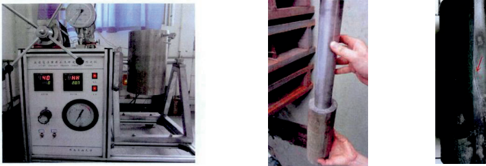
a) Mechanical damage simulation device of cement sheath b) Bonding failure c) Tensile failure
