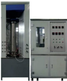
a) Cement sheath integrity evaluation b) The cement sheath sample after the test
