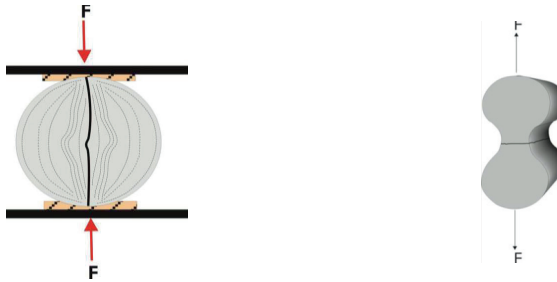
a) Brazil splitting method to test the tensile strength of the cement b) Uniaxial tensile to test the tensile strength of the cement
