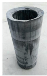
a) Cement sheath integrity evaluation b) The cement sheath sample after the test
