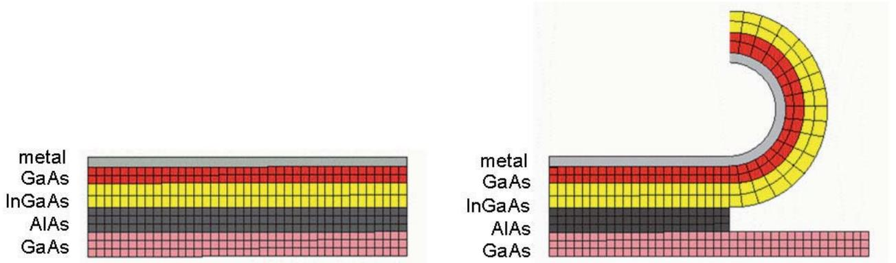
**Figure 2.1:** Principle of the roll up process of a strained metal/(In)GaAs bilayer into a microroll.
