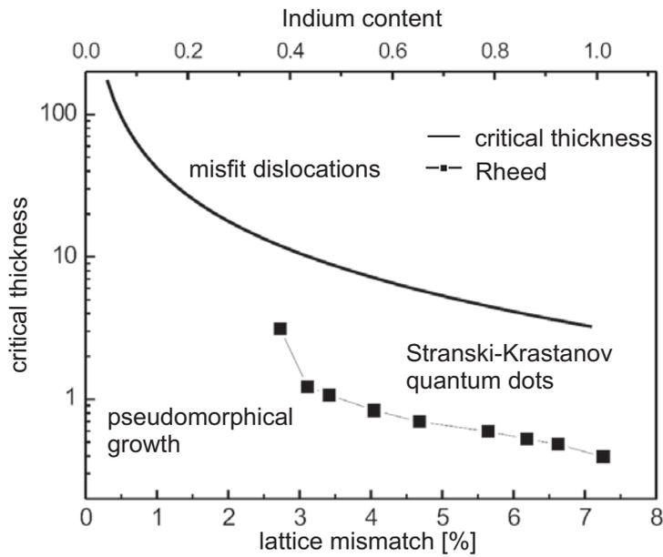
**Figure 2.2:** Phase diagram for the epitaxial growth of strained  $In_xGa_{1-x}As$  on  $AlAs$ . The solid line shows the theoretical curve for the critical thickness with respect to lattice mismatch and Indium content [Mat74]. The phase boundary for Stransky-Krastanov growth (black points) was experimentally measured by Christian Heyn [Hey01].
