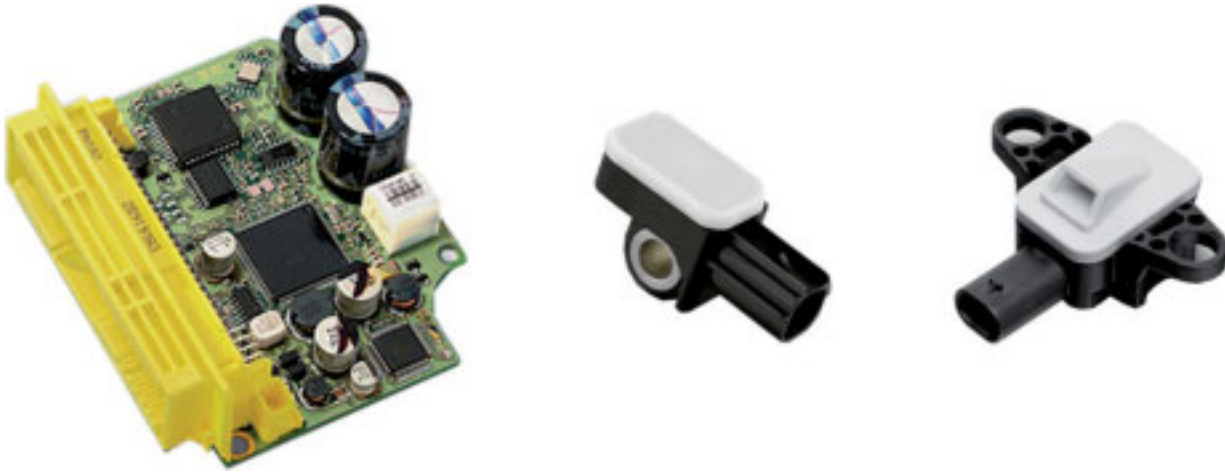
Figure 1.2: ACU (left) and Crash Sensors (right: g-Sat, p-Sat) [3]
