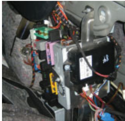
Figure 1.3. Packaging of the electronics in the right rear-end of the Mercedes-Benz E-Class.
