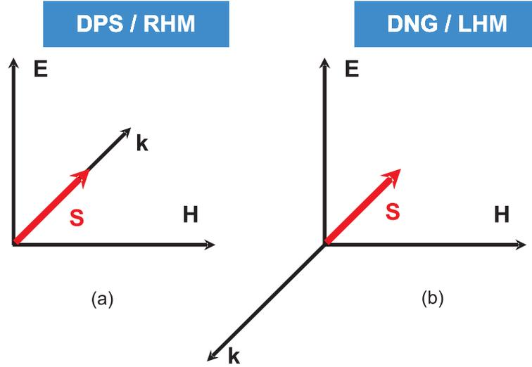
Figure 2.3: Representation of the three vectors  $\mathbf{E}$ ,  $\mathbf{H}$  and  $\mathbf{k}$  for a right-handed medium (RHM) (a) and left-handed medium (LHM) (b).
