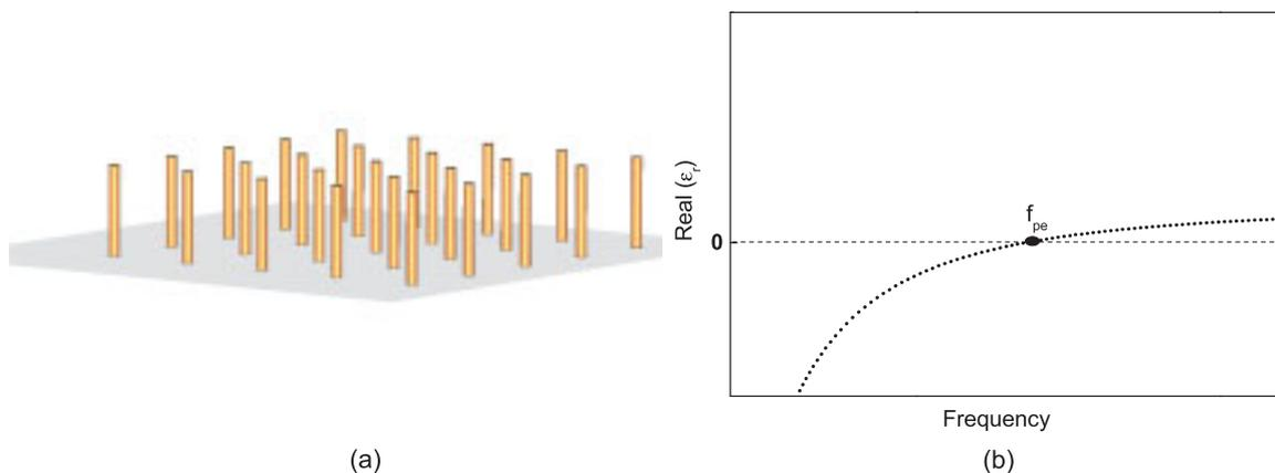
Figure 2.5: (a) Wire medium with an applied electric field along the axes of the wires (b) real part of  $\epsilon_r$  versus frequency.
