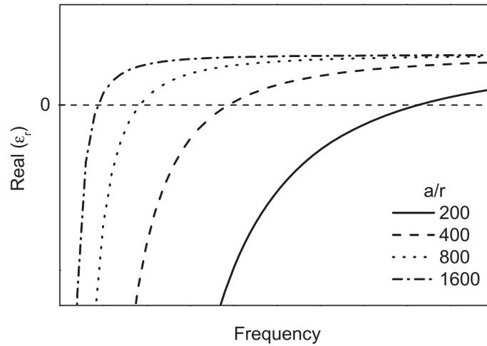
Figure 2.6: Analytical calculation of epsilon for a thin wire medium when  $a/r$  ratio is varied.
