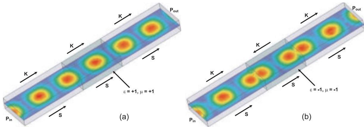
Figure 2.4: Forward- (a) and backward- (b) wave demonstration using a slab of material with  $\epsilon$  and  $\mu$  equal 1 and -1, respectively.
