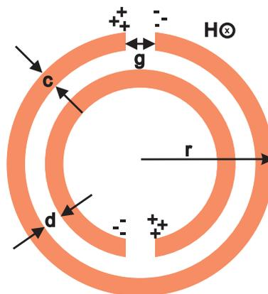
Figure 2.7: Top-view of split ring resonator cylinder structure.
