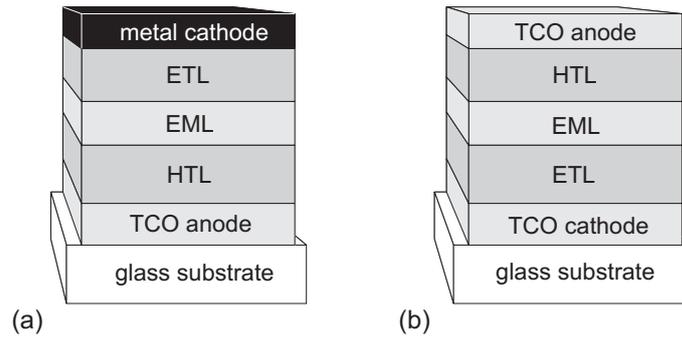
Figure 1.1.: Scheme of a conventional OLED structure (a) and an inverted transparent OLED structure (b).
