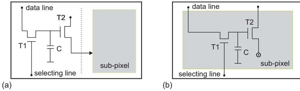
Figure 1.2.: Scheme of an OLED integration on a TFT driver circuit. (a) Horizontal integration. (b) Vertical integration.
