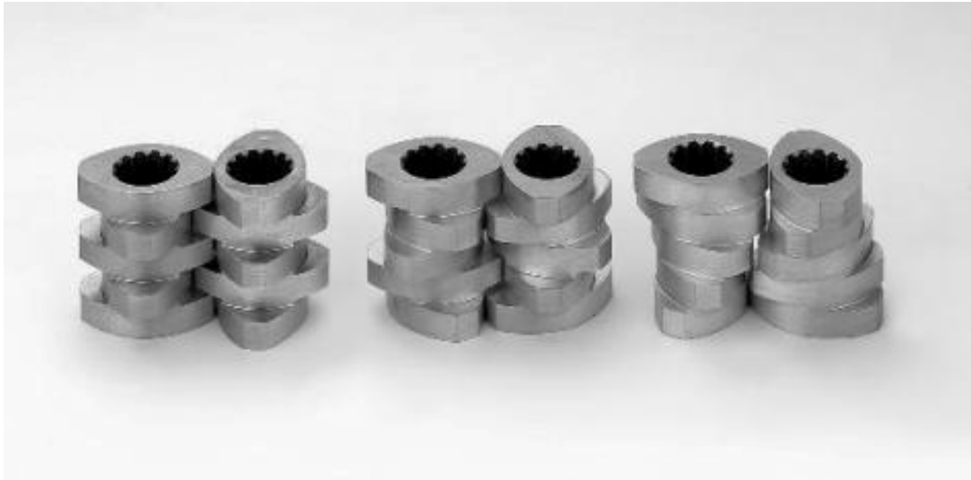
Fig. 2 Kneading blocks of 30mm length with 90°, 60° and 30° advance angle (from left to right)
