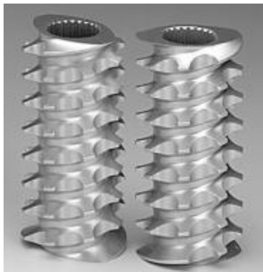
Fig. 3 Combing mixer elements of 60mm length with 15mm element pitch
