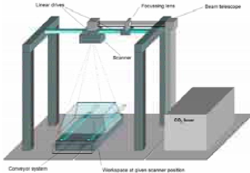
**Figure 2.2:** Structure of a typical CO<sub>2</sub> laser remote welding system
