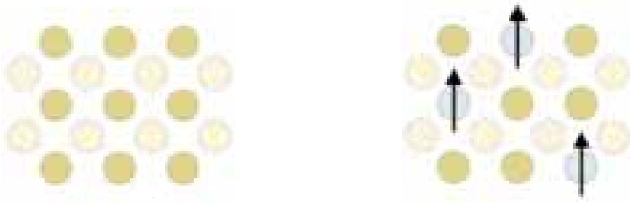
Figure 2.1: A nonmagnetic polar semiconductor (left) can be converted to a DMS (right) after diluted incorporation of magnetic ions (i.e., ions bearing a net magnetic moment) in the host lattice.
