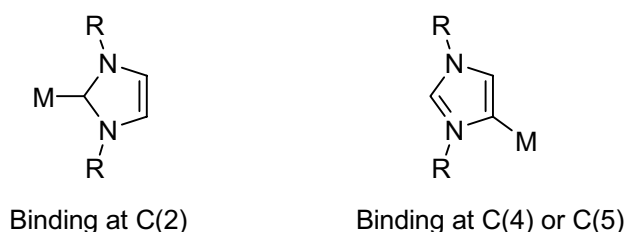
Figure 1.8 C(2) and C(4) or C(5) binding mode of the NHCs.
