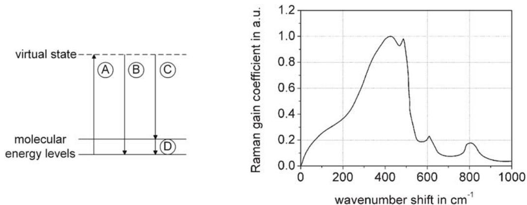
Figure 1.3: Energy diagram of RFA and Raman gain coefficient of the SiO<sub>2</sub> fiber
