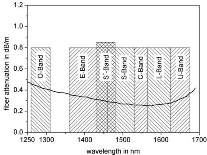
Figure 1.1: The normalized ITU bands for optical transmission systems
