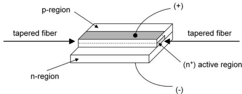
Figure 1.2: Schematic diagram of an SOA
