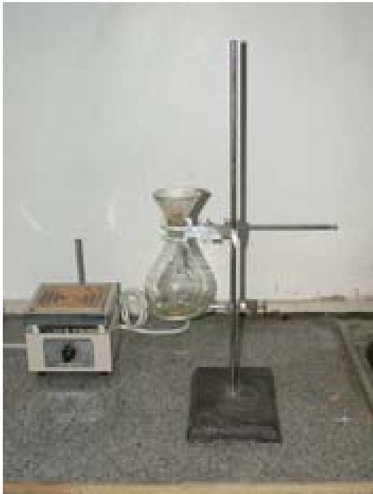
Fig.4: Removal of unreacted NaH by filter paper to stop Abamectin activation reaction
