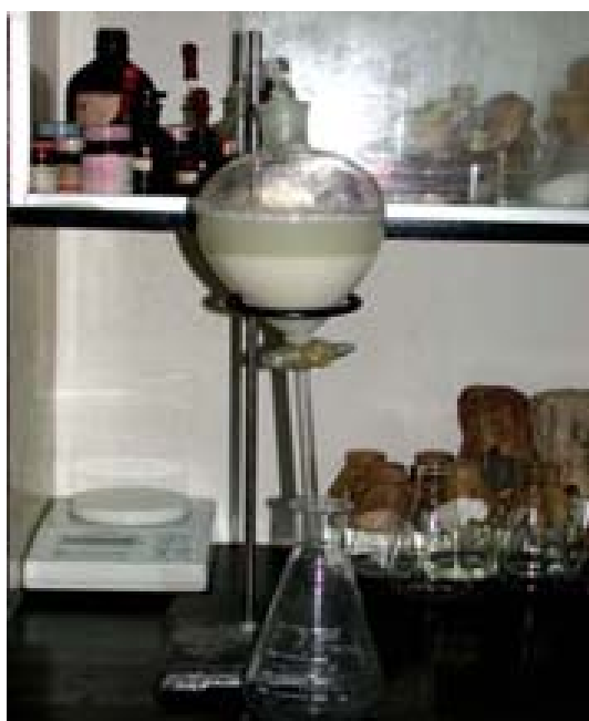
Fig. 2: Two-phase liquid method for B.t. toxin crystal purification (The upper layer was B.t. toxin crystal)
