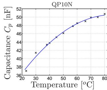
Figure 1.2: Measured temperature dependency of the piezoelectric capacitance.
