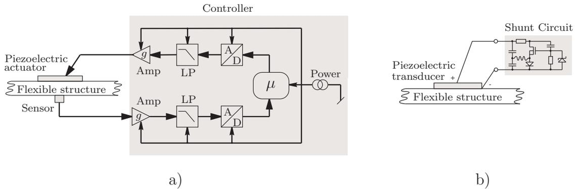
Figure 1.3: a) Conventional vibration control and b) the piezoelectric shunting technique. The latter approach is described in the present thesis.
