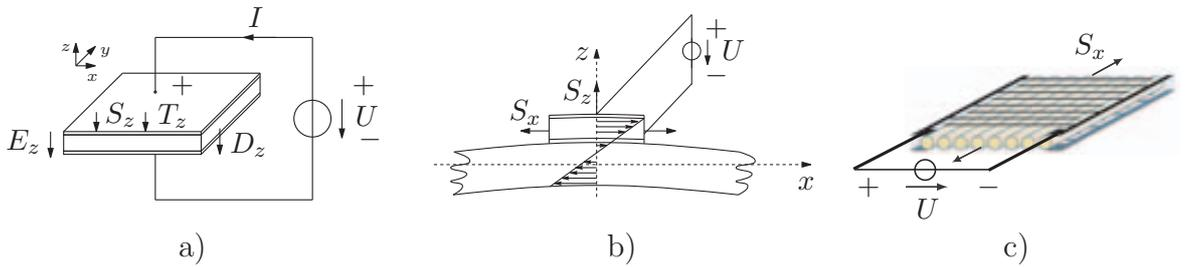
Figure 1.1: a) Piezoelectric stack actuator. b) Piezoelectric transducer on a mechanical structure. Due to the applied voltage  $U$ , the transducer bends the mechanical structure. c) Integrated piezoelectric fiber composite structure.
