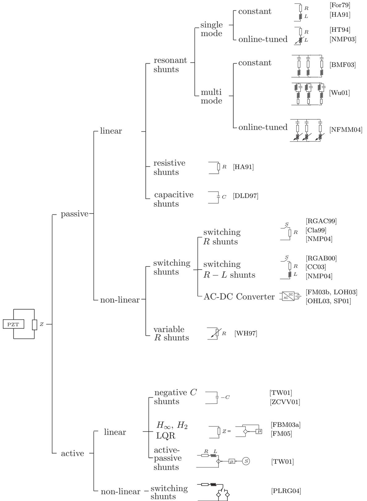
Figure 2.1: Different topologies of shunt networks for shunt damping
