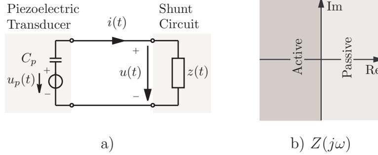
Figure 2.2: Definition of passive and active shunts: a)  $z(t)$  shunted to the piezoelectric transducer. b) Passive and active impedance  $Z(j\omega)$  in the frequency domain.
